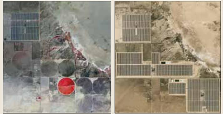
Areal imagery of the Harper Lake area showing center pivot farms in 2007 (left, near infrared false-color image) that were converted to solar fields by 2015 (right). Land-use changes such as those illustrated above require less water and may help explain some of the water-level recovery observed in this area. Images provided by Mojave Water Agency (used with permission).
